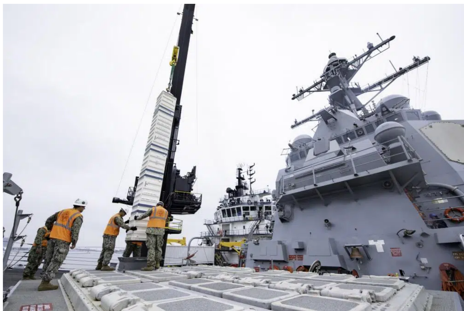
Sailors aboard Arleigh Burke-class guided-missile destroyer USS Spruance (DDG 111) guide training ordnance into the ship's forward vertical launch system (VLS) cells during a proof-of-concept evolution in San Diego. Oct. 4. MV Ocean Valor conducted its first at-sea vertical launch system reload with Spruance, demonstrating the ability of the U.S. Navy to re-arm surface vessels who employ VLS. (U.S. Navy photo)
