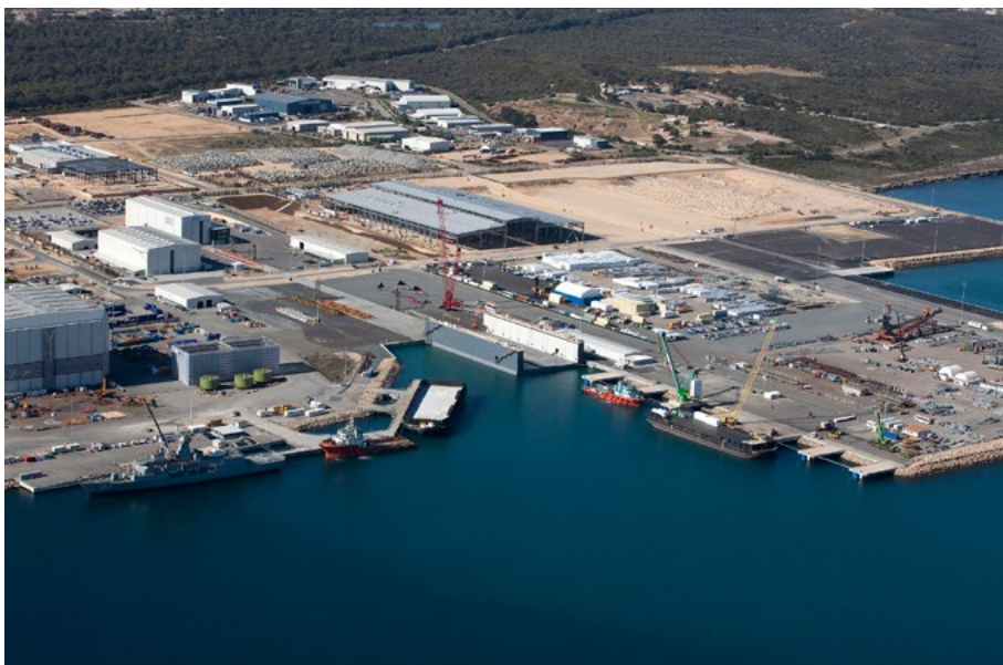
ASC's other facility is at Henderson, Western Australia, seen here from the air. The ship lift used to raise submarines onto hardstands for maintenance work is in the centre of the photo. (Photo courtesy ASC).
